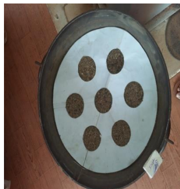
Fig 2: Marking of reinforcement location
